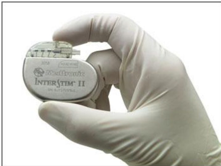
Figure 1: The permanent stimulator that is implanted under the fat in the buttock. The temporary stimulator is larger and worn on your belt during the test period.
